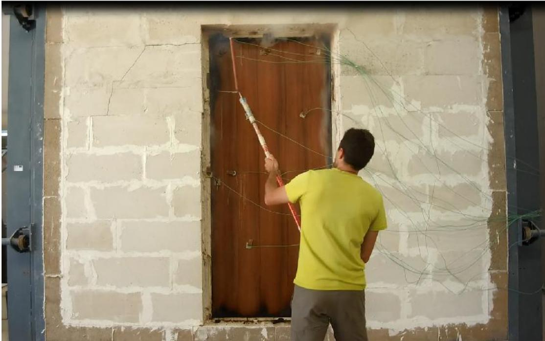
**Fig. 9 Gap gauge check: the 6 mm gap gauge can be passed through the test specimen such that the gauge projects into furnace (but cannot be moved a distance of 150 mm along the gap) at 1h 12 min post the commencement of the test**
