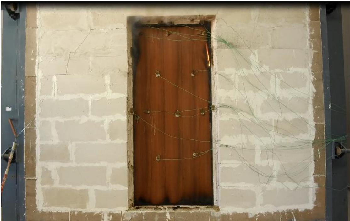
**Fig. 10 Sustained flaming (continuous flame lasting more than 10 s) at 1h 19 min post the commencement of the test**
