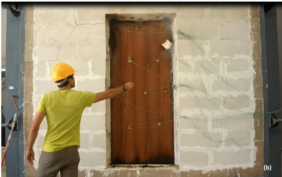
**Fig. 8 Cotton pad check: (a) 1h (cotton pad remained intact) and (b) 1h 19 min post the commencement of the test (cotton pad ignition)**
